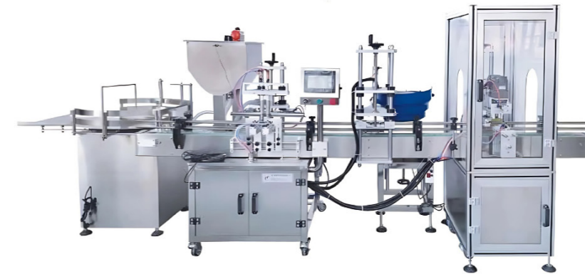
Six - head self - low filling machine + Automatic drop cover + Automatic rubbing machine
